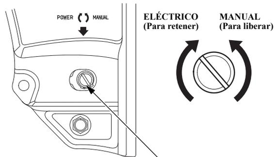
**VÁLVULA DE DESCARGA MANUAL**
