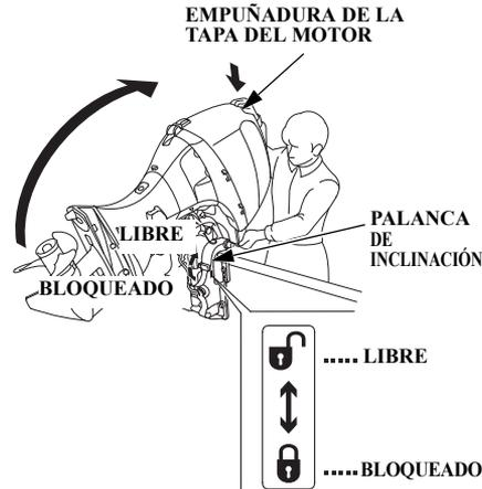
2. Move the tilt lever to the FREE position. Hold the engine cover grip and raise the outboard motor. (The outboard motor can be tilted stagelessly.)
